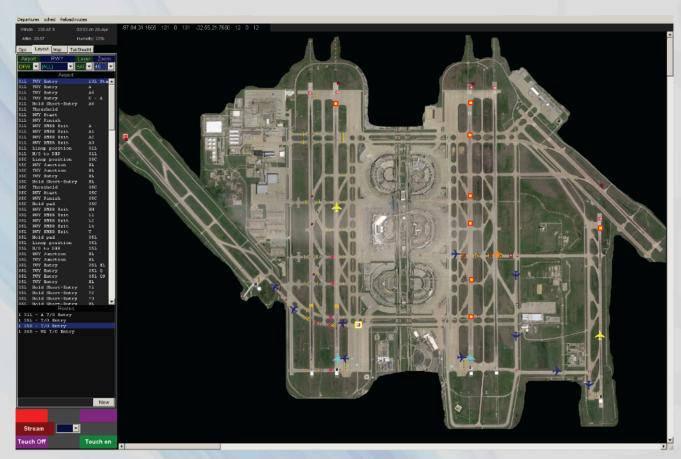
**AAATCS** can also operate as a primary or backup remote tower, providing ANSP's with multi-tower functionality on a controller working position.
