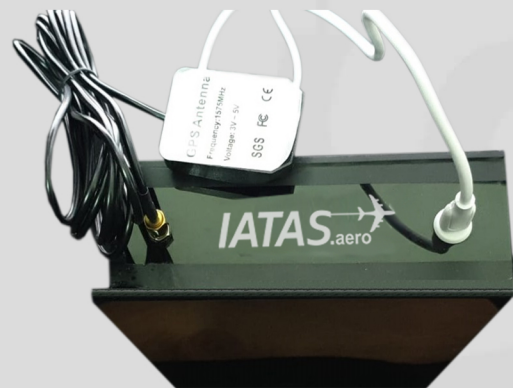
Vehicle tracking unit with all weather airport moving map for situational awareness and pre-incursion alerts
