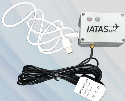
Vehicle unit with GPS location and pre-incursion alert, over GSM/WiFi
